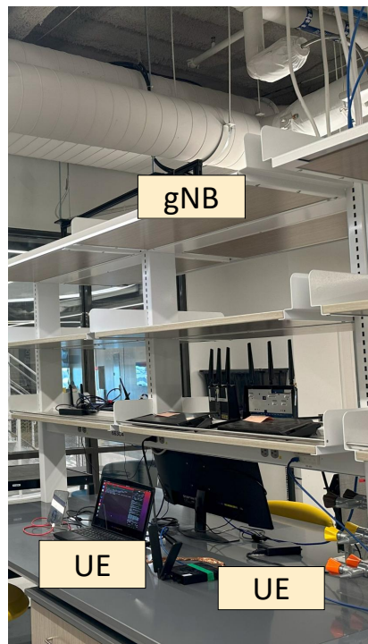
(a) OTA setup used in our experiments.
