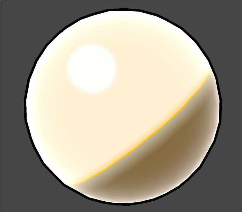
Figure 14. Draw the outline by extending it outward from the normal direction (either two passes on one material or two materials), position = position + normal * 0.01 , cull front
