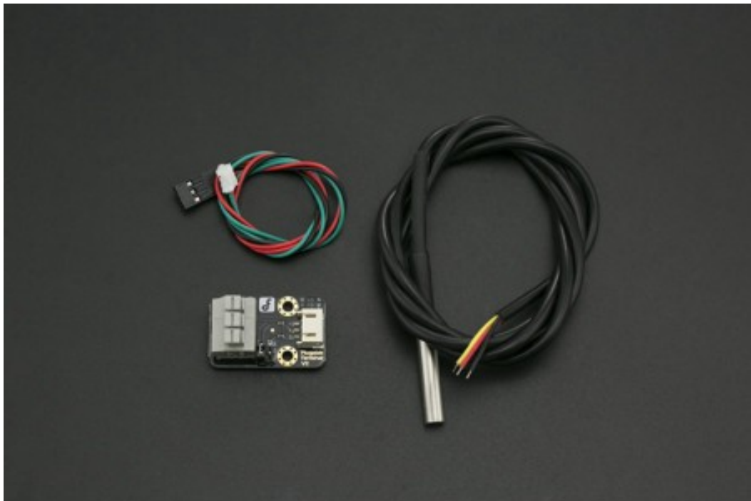
Figure 2.3. Waterproof DS18B20 Digital Temperature Sensor
