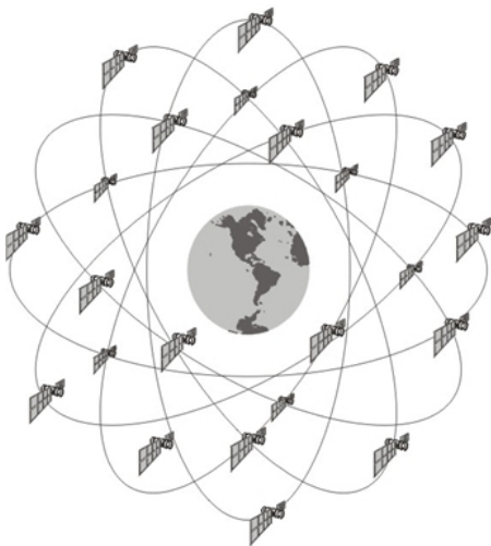
21 SATELLITES WITH 3 OPERATIONAL SPARES, 6 ORBITAL PLANES, 55 DEGREE INCLINATIONS 20,200 KILOMETER, 12 HOUR ORBITS
