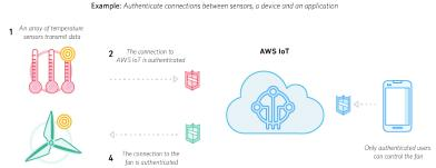
If the sensors agree the temperature is above a threshold they turn on the fan
