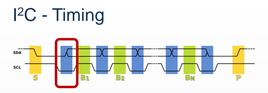
2. SCL is pulled low, and SDA sets the first data bit level while keeping SCL low (during blue bar time).
