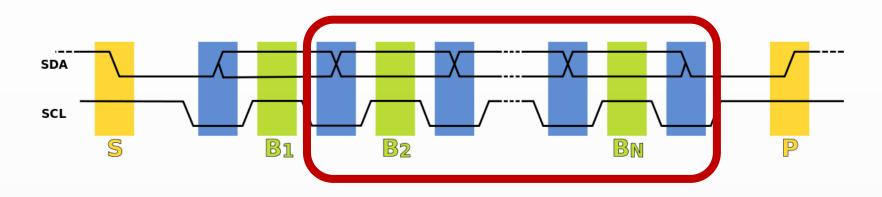
4. This process repeats, SDA transitioning while SCL is low, and the data being read while SCL is high (B2, ...Bn).
