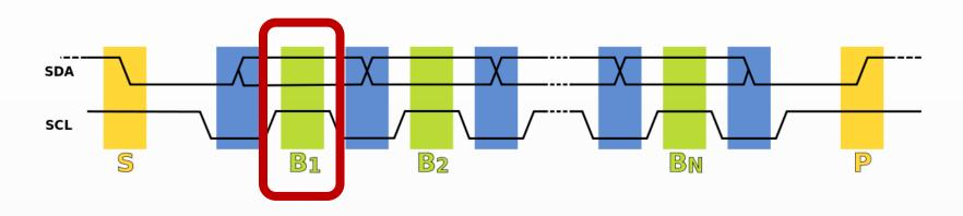
3. The data are sampled (received) when SCL rises for the first bit (B1). For a bit to be valid, SDA must not change between a rising edge of SCL and the subsequent falling edge (the entire green bar time).
